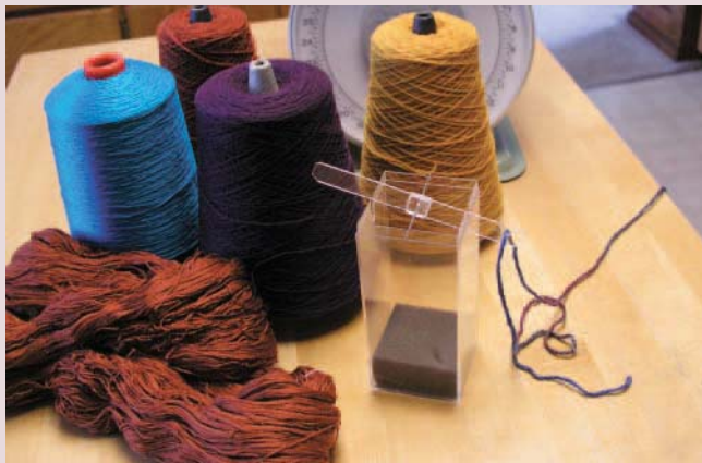
a. Place a strand of the unknown yarn in the triangle of the balance (let the yarn hang off the edge of table or counter).
